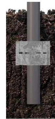
Installation with additional support element - slab
